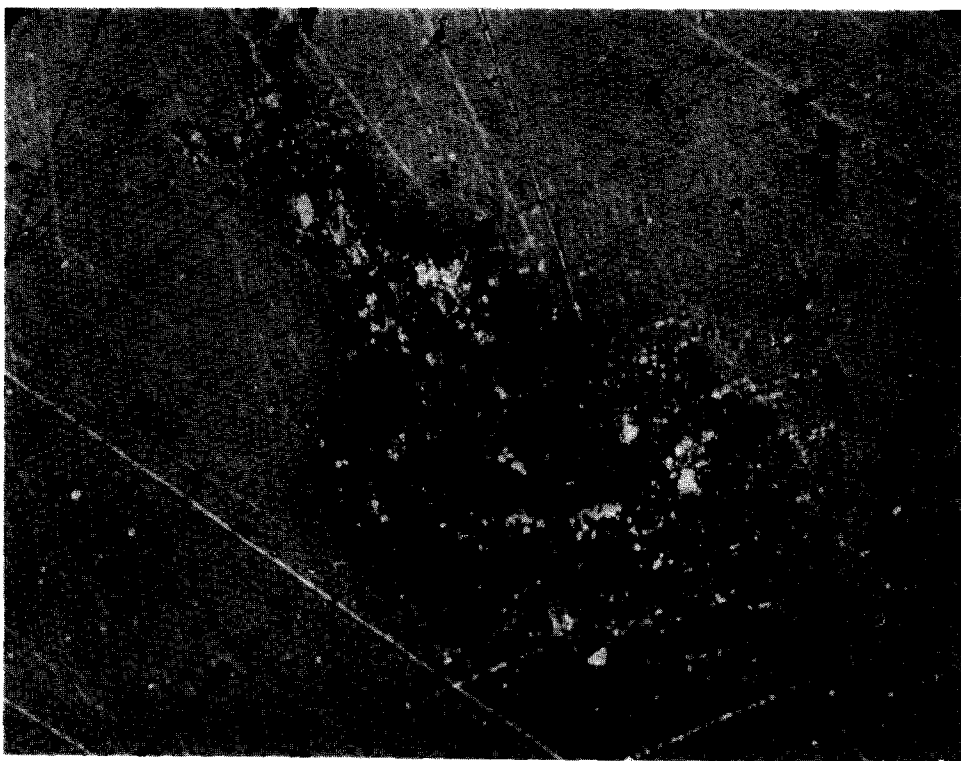
FIG. 4. Copper deposited on a silicon surface in the reaction with copper(I) chloride vapor. The surface consists mainly of free copper, although some \eta phase is also present (white spots). Magnification \times 300 . Polarized light.
